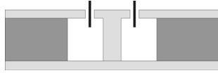
Figure 2 Magnetic system of electro dynamic loudspeaker, the dark areas is the permanent magnet, the gray areas the iron parts of the system, and the black areas is the voice coil placed in the air gap of the magnetic system.
